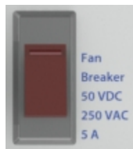
Figure 13. Fan Power Breaker
