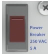
Figure 14. Power In Breaker
