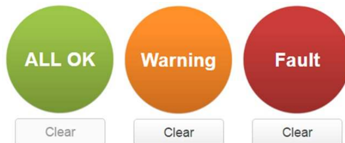
Figure 5. Three possible Nuvation BMS safety states
