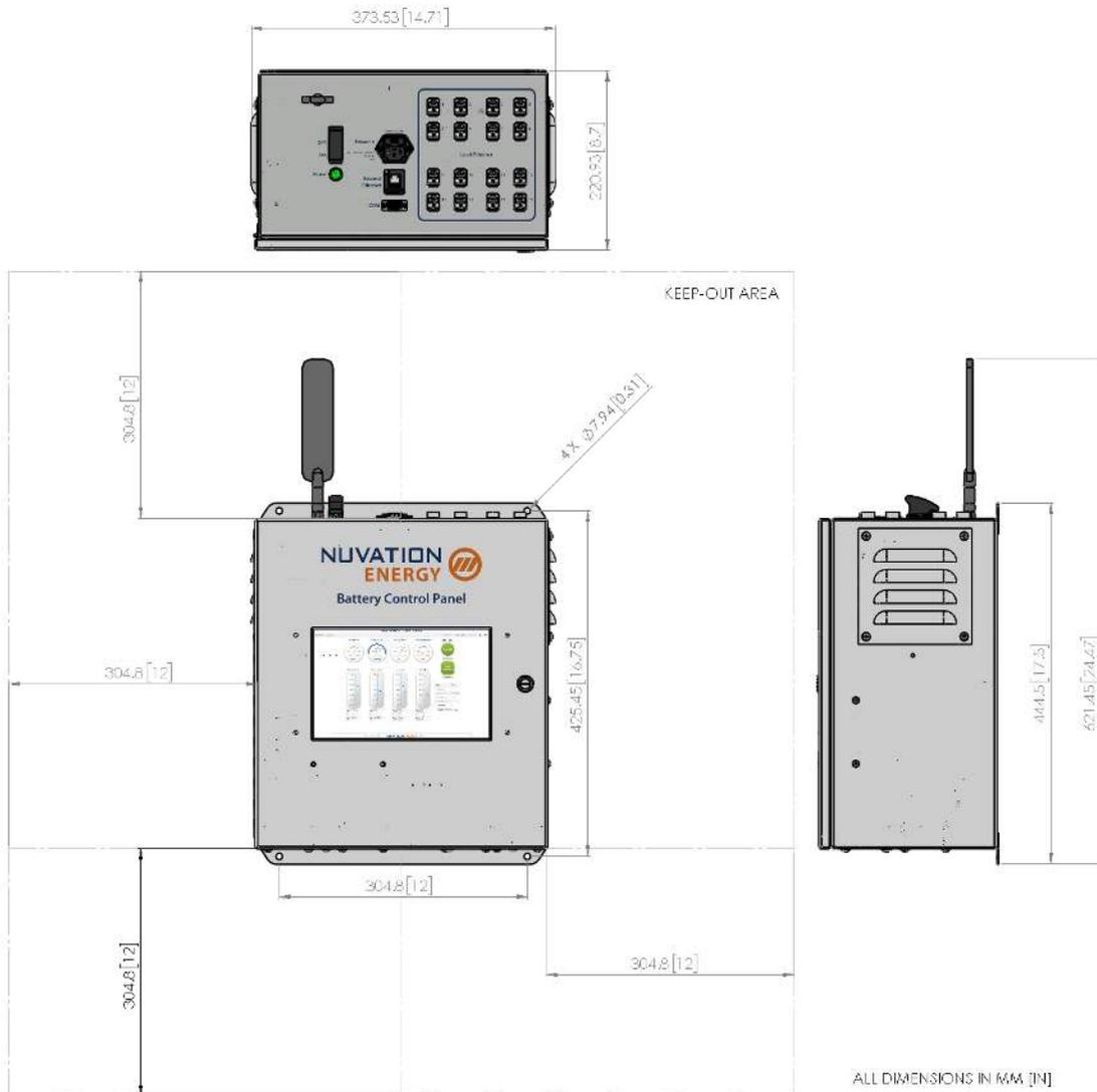
**Figure 4. Nuvation Energy Battery Control Panel Dimensions**
