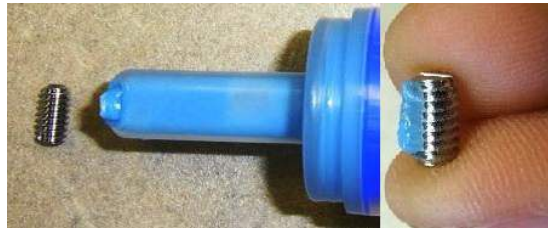
Figure 7. Applying thread locker to set screw
