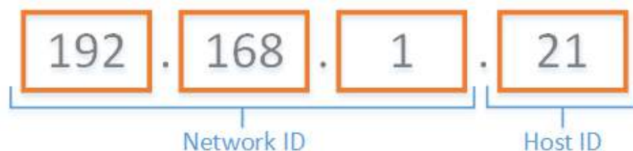
Figure 41. Parts of an IP address
