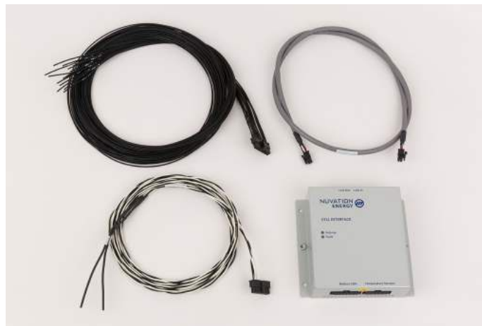
Figure 17. Example Cell Interface kit (NUV100-CI-16-KIT-2)
