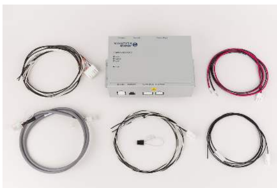
Figure 31. Example Power Interface kit contents
