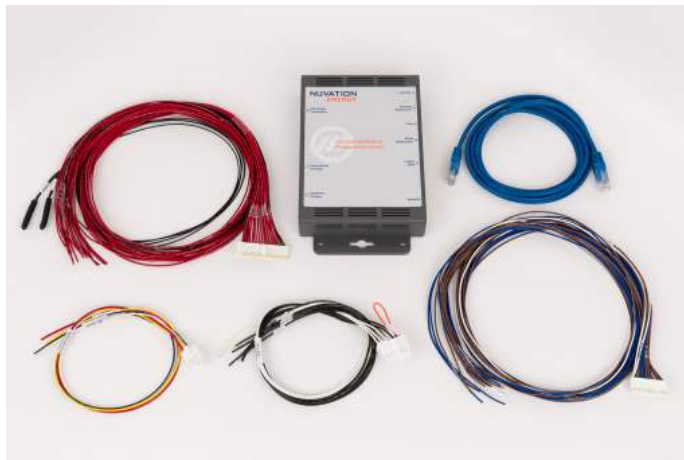
Figure 6. Example Low-Voltage BMS kit (NUV300-BC-16-KIT)
