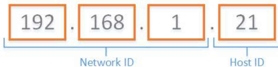
Figure 20. Parts of an IP address
