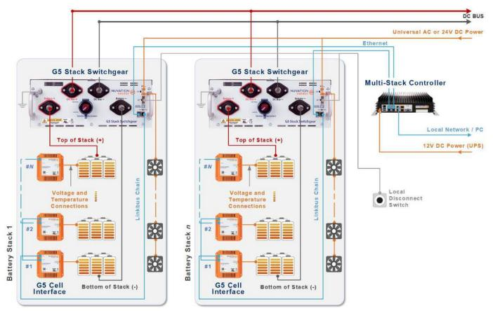
Figure 3. G5 High-Voltage BMS multi-stack diagram
