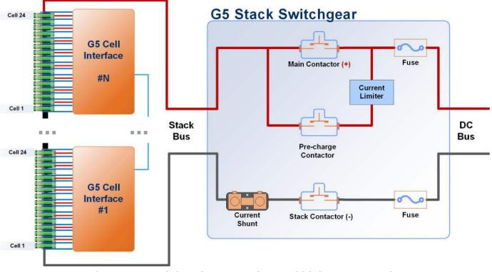
Figure 5. G5 High-Voltage BMS internal high-current path.
