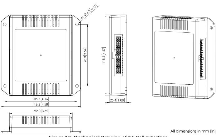
Figure 13. Mechanical Drawing of G5 Cell Interface
