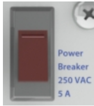
Figure 14. Power In Breaker
