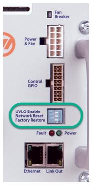
Figure 40. Config Switches
