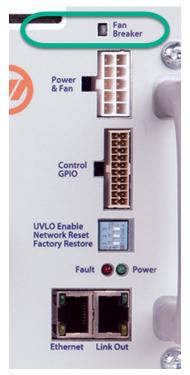
Figure 33. AC Fan Breaker
