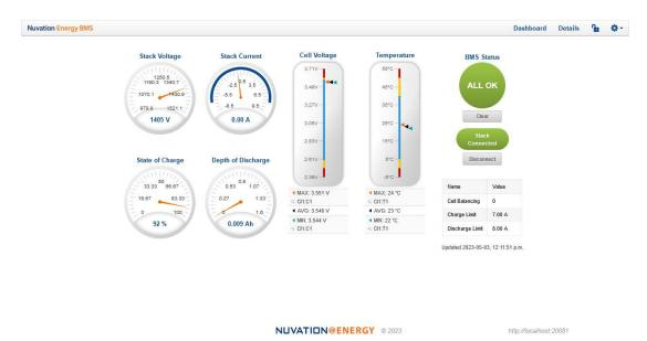
Figure 47. Nuvation Energy BMS Operator Interface Dashboard screenshot
