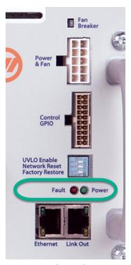
Figure 45. Fault and Power LEDs
