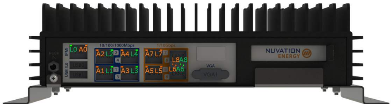
Figure 13. Multi-Stack Controller Port LEDs
