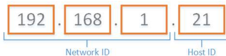
Figure 42. Parts of an IP address
