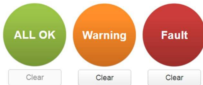
Figure 62. Three possible Nuvation Energy BMS operation states
