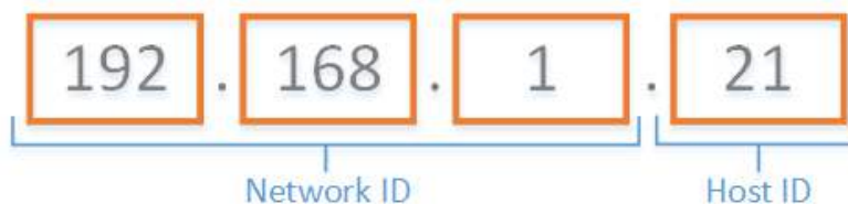
Figure 42. Parts of an IP address
