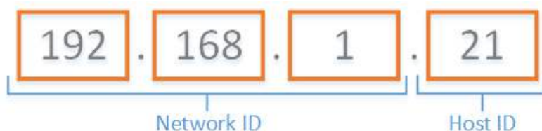
Figure 45. Parts of an IP address
