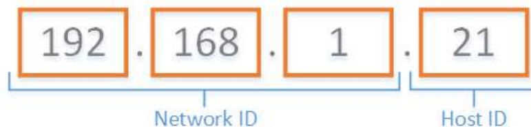
Figure 39. Parts of an IP address
