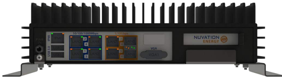
Figure 5. Multi-Stack Controller external interfaces (front)
