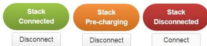
Figure 66. Three Nuvation Energy BMS Operating States
