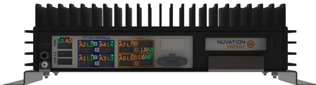
Figure 13. Multi-Stack Controller Port LEDs
