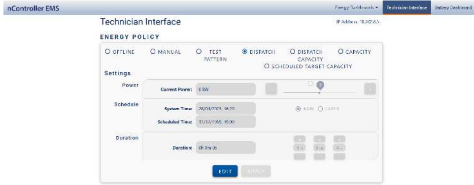
Figure 20. Technician Interface Dispatch Policy
